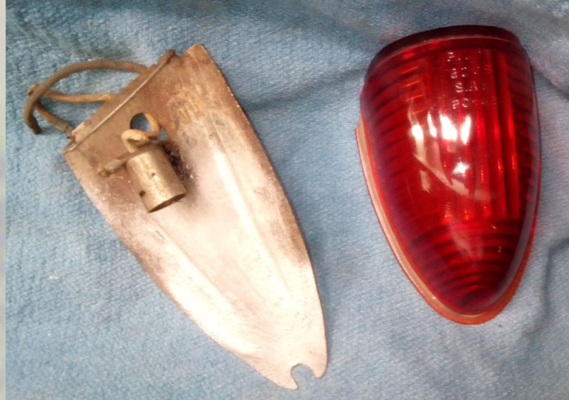
Glass Red Marker Lens and backing plate with bulb holder Fits GM - Old Look
