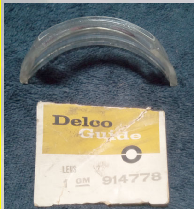
Clear Glass Lens GM 914778 for License Plate Lens
