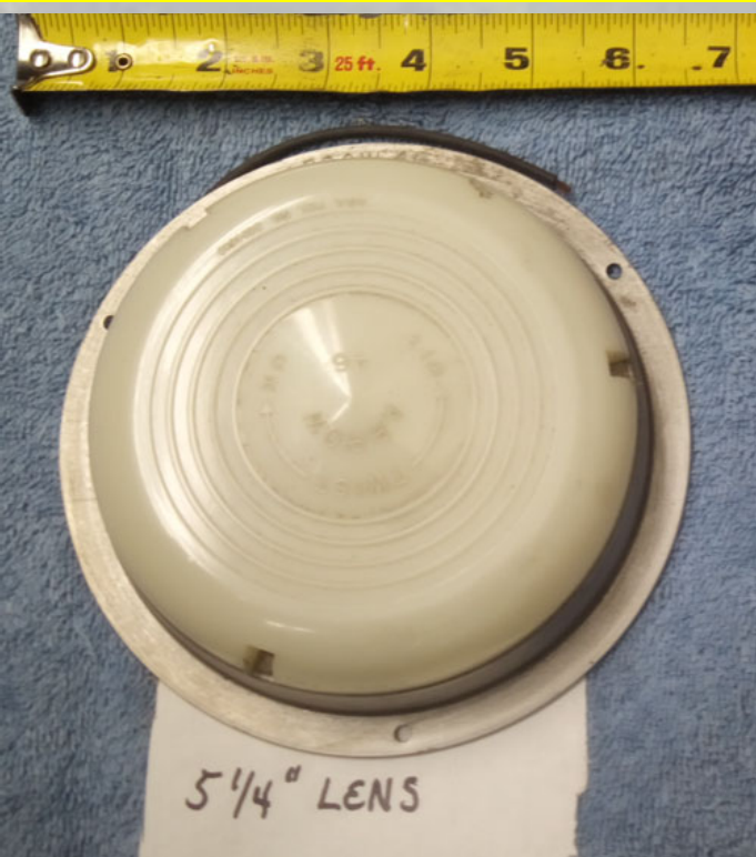
Clear Dome or Courtesy Light Assembly, 3 3/4 inch housing diameter, GM9 stamped on housing
