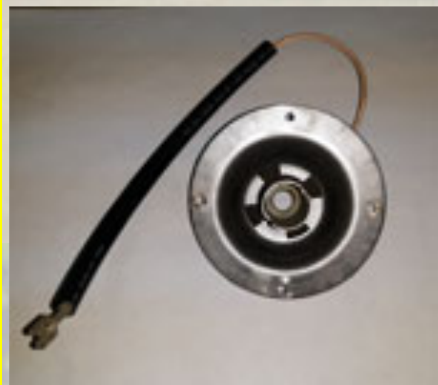
Round Clear Back Up Lens SAE-R-73 Lens GM 5961260, socket assembly, plastic rings, chrome metal rings
