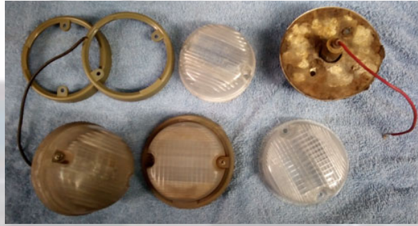
Round Clear Back Up Lens SAE-R-73 Lens GM 5961260, socket assembly, plastic rings, chrome metal rings
