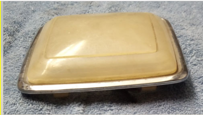
White Dome Light Assembly, 4 1/2 inches square
