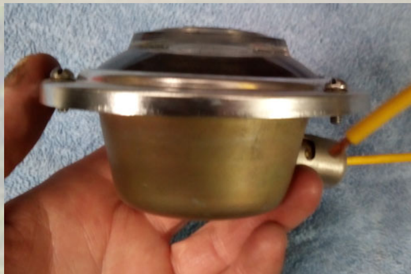
Clear Dome or Courtesy Light Assembly SAE-P1-68, 4 1/2 inch diameter housing
