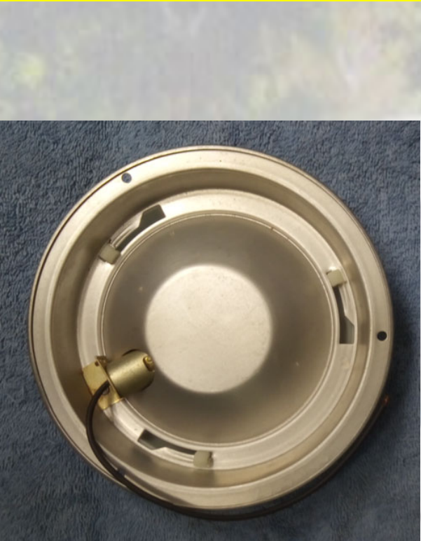
Clear Dome or Courtesy Light Assembly, 3 3/4 inch housing diameter, GM9 stamped on housing
