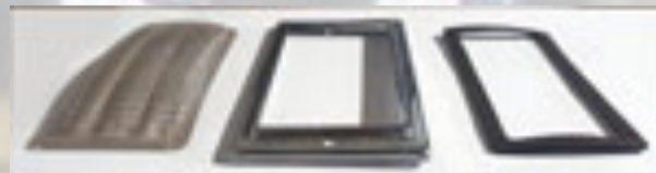
Lavatory Dome Lens Trim and Gasket
