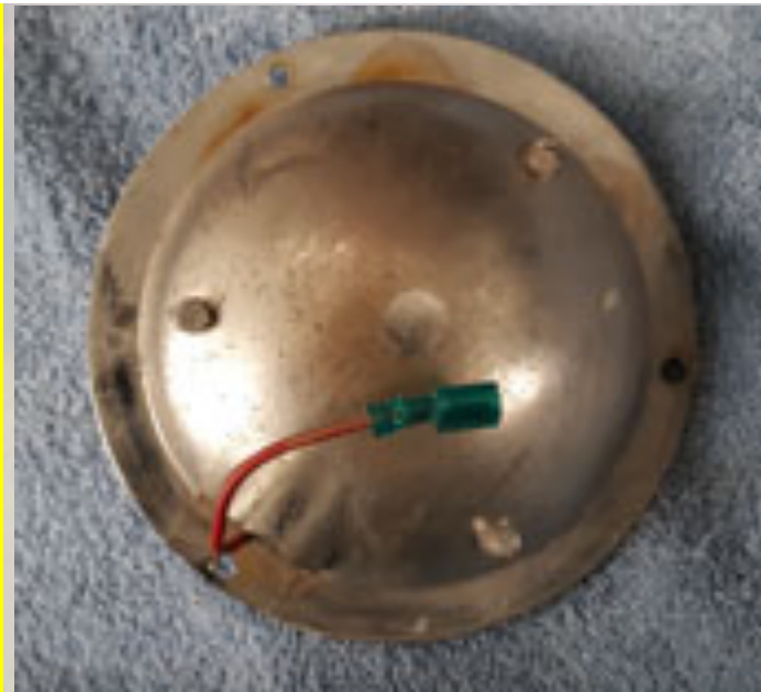
Round Amber Marker Assembly 4.25 inch lens diameter
