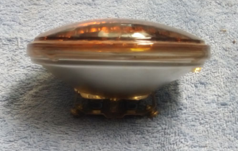
Round Amber Headlight, GE 4414R, 4.25 inch diameter.
