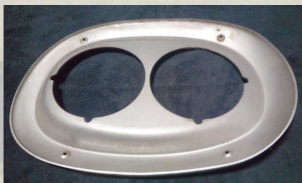
Chrome Round Double Headlight Bezel or Trim. 5961890 stamped on rear, in excellent condition for MCI, 5.75 inch diameter
