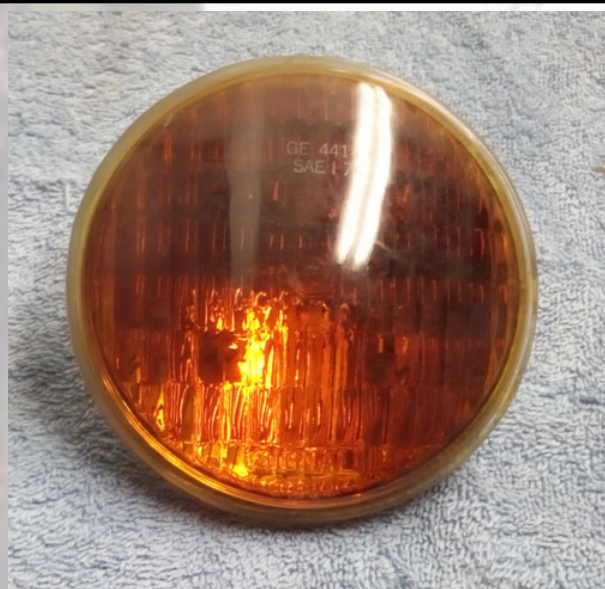
Round Red Headlight, GE 4414R, 4.25 inch diameter
